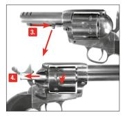
Rotate cylinder until a cartridge is centered in the loading gate. 3. Pull back cartridge ejector. 4 Cartridge is ejected.
